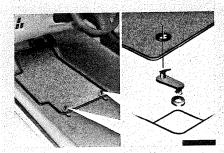
Secure the driver's floor mat using the hooks provided.
